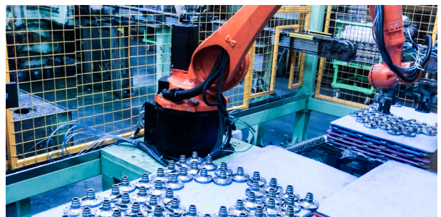
Vision-Guided Compressor Bearing Loading
