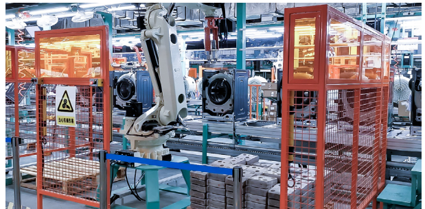
Vision-Guided Counterweight Loading
