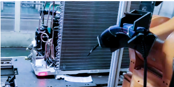
Vision-Guided AC Halogen Leak Detection
