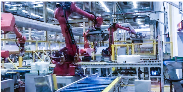
Vision-Guided Washing Machine Drum Loading
