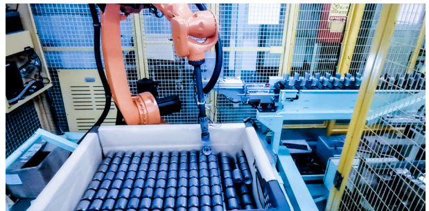
Vision-Guided Compressor Rotor Loading
