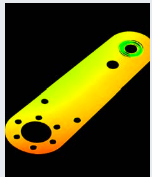
Metal plate flatness inspection
