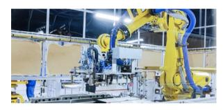
**Vision-Guided Machine Tending of Battery Modules**
