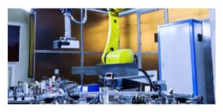
**Inline Measurement of Bumper Beams**
