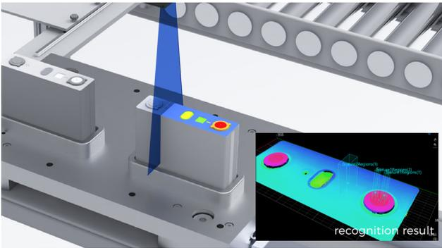
Dimensional measurement (battery cell cap)
