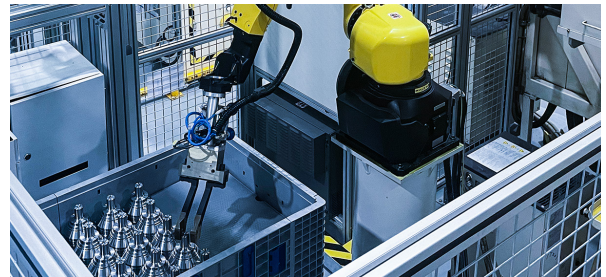
Vision-Guided Bin Picking of CV Joints
