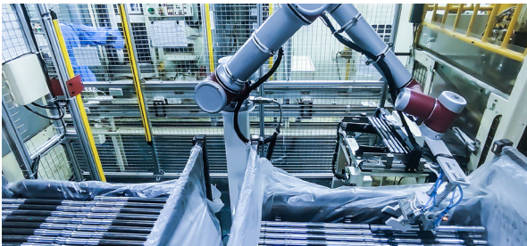
Vision-Guided Machine Tending of Countershafts
