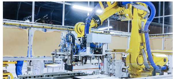
Vision-Guided Machine Tending of Battery Modules
