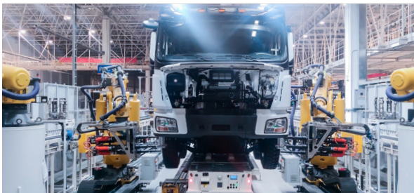
Vision-Guided Heavy-Duty Truck Tire Assembly
