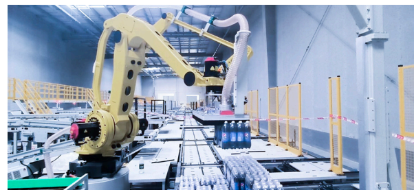
Vision-Guided Depalletizing of Shrink-Wrapped Bottles
