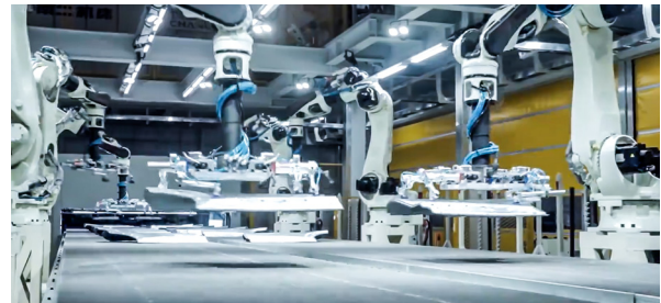
Vision-Guided De-racking of Stamping Parts
